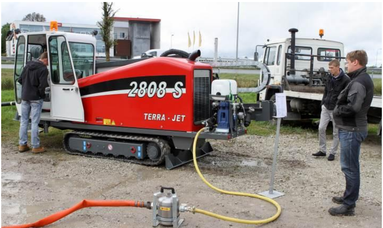
Pic. 4: The TERRA-JET TJ 2808 S can be adapted with an air percussion head.
