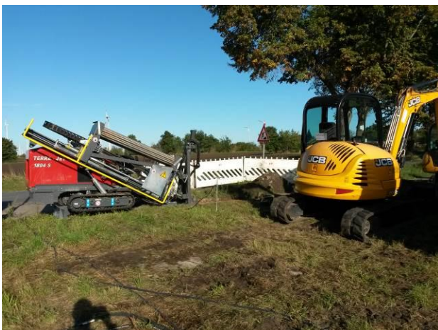
Bild 6+7: The TERRA-JET in drilling position. Due to the extreme entry angle of up to 67% the required drill depth could be reached immediately. The anchoring with the two ground anchors is fast and easy.
