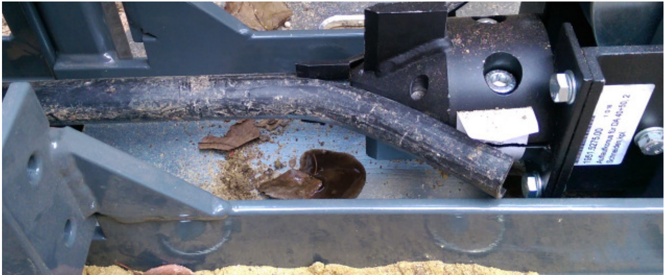
Pic. 4: During bursting, the old PE pipe is regularly pushed out of the ground into the cable burster. This is why the TERRA-EXTRACTOR X 100 can be equipped with a swell cone which cuts the old pipe into two halves. This prevents a shrinking of the old pipe.
